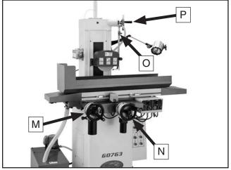
Figure 4. Handwheel controls.
